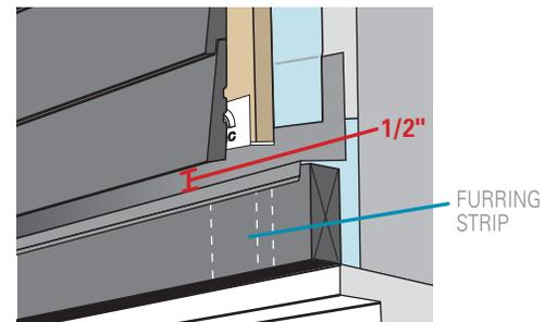
1/2" space between the siding and the flashing over all openings
