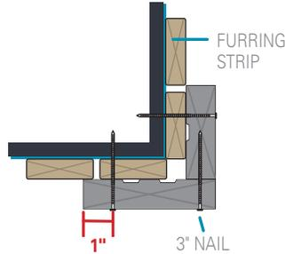
**!** NEVER JOIN TWO PIECES OF SIDING CUT AT A 45° ANGLE TO MAKE CORNERS. THIS WILL LIMIT YOUR OPTIONS FOR MAKING ADJUSTMENTS DURING INSTALLATION. THE SHIFTS THAT OCCUR NATURALLY IN WOOD WILL ALSO BECOME MORE NOTICEABLE OVER TIME. [FIGURE 38]
