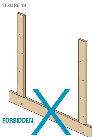
**NEVER INSTALL FURRING STRIPS DIAGONALLY, WHICH WILL IMPEDE VENTILATION OF THE WALL AND PREVENT WATER FROM DRAINING FREELY. NEVER INSTALL FURRING STRIPS HORIZONTALLY AT THE BOTTOM OF WALLS OR AROUND DOORS AND WINDOWS. [FIGURE 18]**
