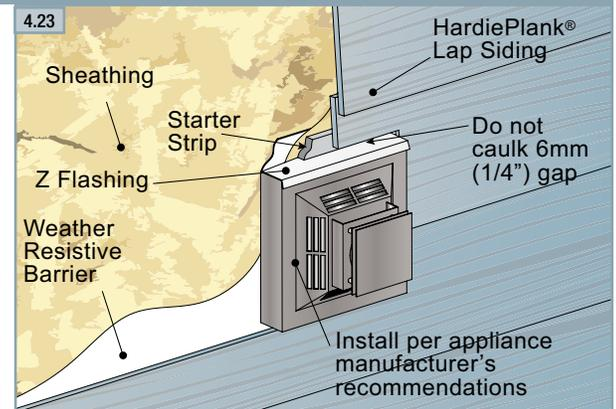
For dryer vents, avoid placement too low to the ground where debris could easily impede air flow, trapping heat and moisture. Some types of high efficiency furnaces can be vented out through the walls. In these cases, avoid locating the vent too close to the roof or eaves where heat and moisture will be trapped.
