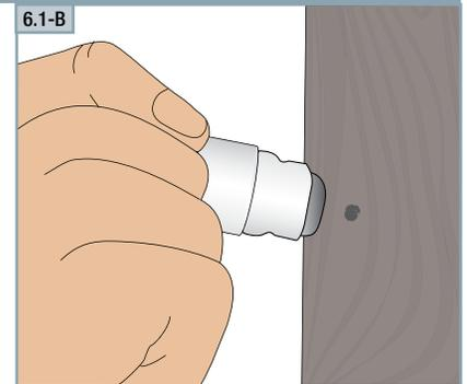
**Touch-up Pens** - conceal nailheads and very small nicks and scratches less than a dime size. Replace the area with a new piece of plank or panel if area is larger than a dime.
