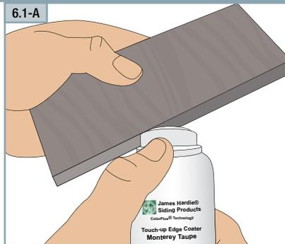
**Edge Coater** - edge coating is required for any field cuts to seal the edges and make joints less visible.
