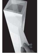
Christy's Red Hot or TrimWelder White Hot are a few recommended solvent based PVC adhesives. Do not use thick 2-component adhesives. They will fracture the miter corners. PVC glue softens the joint of the VERSAWRAP reducing cracking of the cellular PVC at the outside corners of the wrap. Remember to apply the adhesive to only one surface of the miter lock joints. **NOTE:** Four VERSAWRAPS can be glued using one 5 ounce tube of Weld-On 705 regardless of column length.
