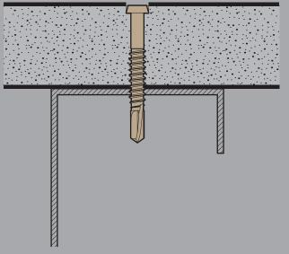
Note: Wings on 15%" Deckfast Metal are designed to shear off during installation.
